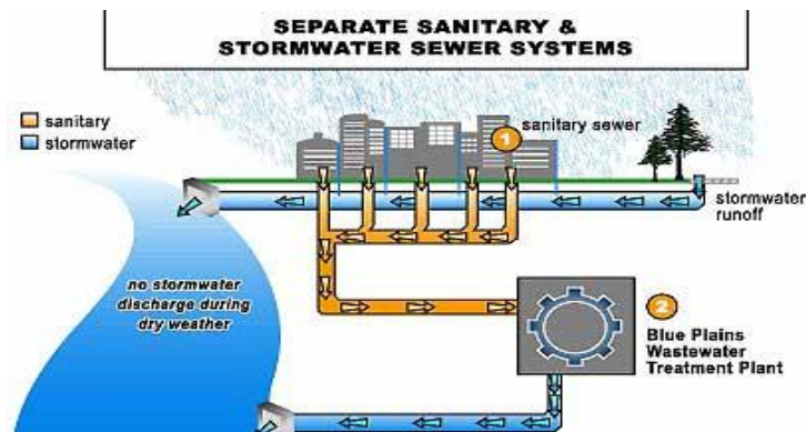
Figure A. Combined vs. separate sewer systems and storm drains
